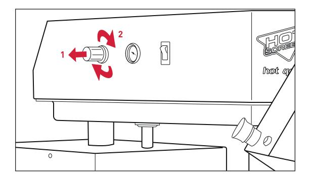
HOT 4000 is equipped with a pressure regulator and a manometer to read the pressure in the internal compressed air system.
